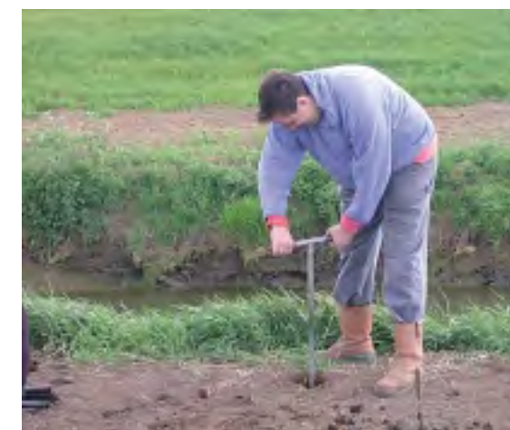
Jim Williams installing piezometers at Fiskerton. Note sections of the wooden causeway visible just below and slightly left from Jim's right hand. Photograph: Vanessa Fell
