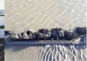
Frames sticking out of the water with treenails connecting them to the outer planking. Credit: MSDS Marine
