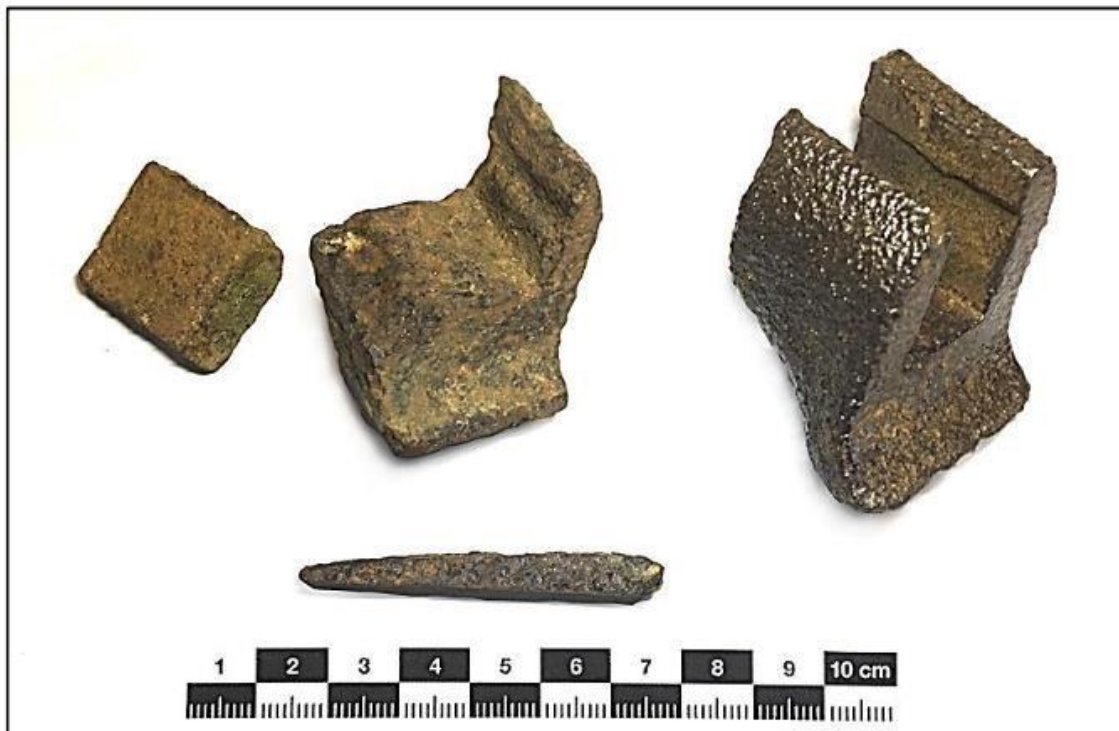
Batten cleats. Illustrated inverted – legs face down in operation. LEFT: small style with broken leg, RIGHT: large style unbroken, LOWER: wedge used to secure cleat to rafter.
