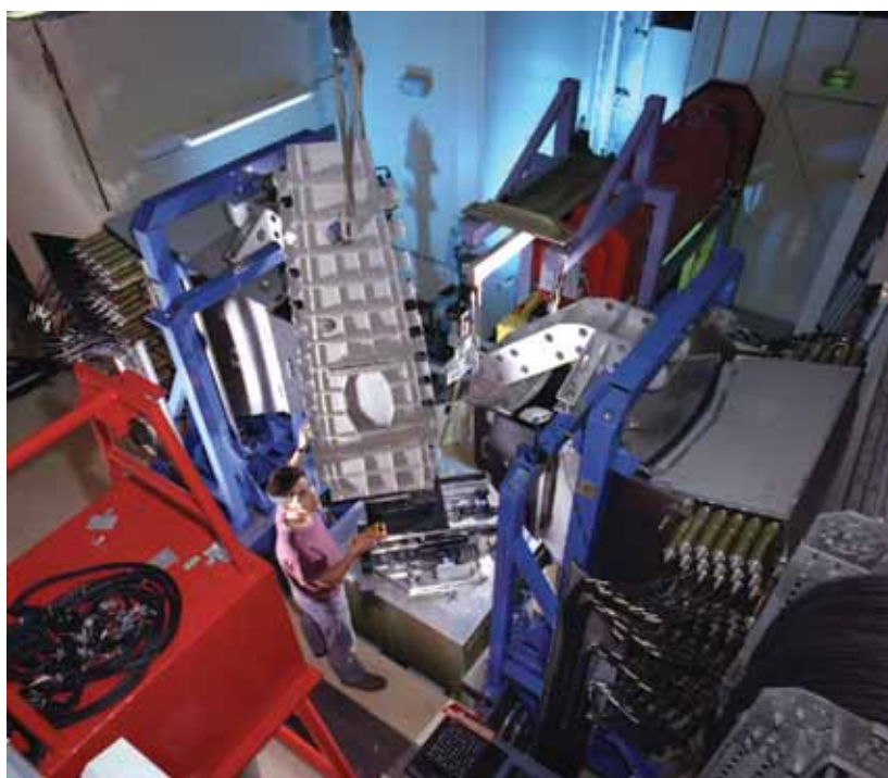
The sample stage on the ENGIN-X neutron diffraction beamline at ISIS is big enough to do non-destructive microstructural analysis of whole, intact archaeological objects (or an airplane wing spar as shown here). Photograph: Stephen Kill
