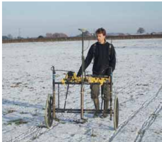
The Foerster Ferrex in use in Shropshire with GPS positioning integrated into the data collection. The three sensors are visible on the frame
