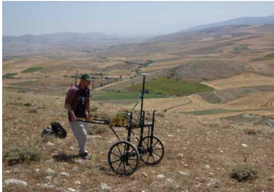
The Foerster Ferrex in use in Turkey with GPS positioning
