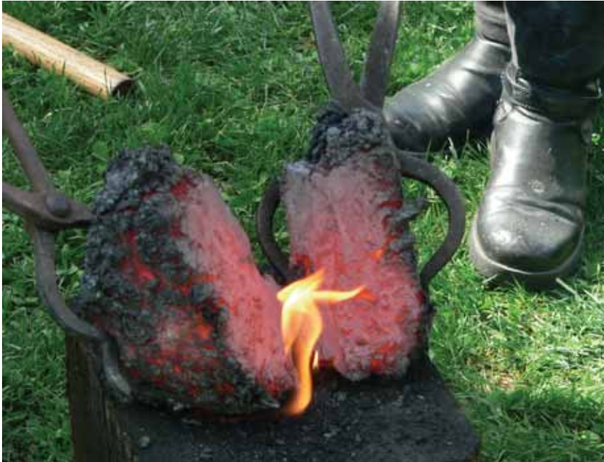
Bloom straight out of an experimental furnace, split with an axe
