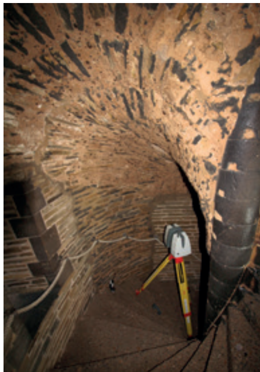
Laser scanning within the interior of the gatehouse at Newark Castle
